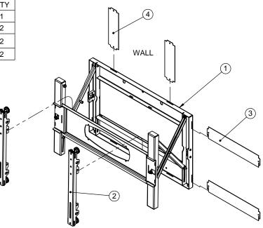
**WARNING**: Ensure the structure that you are attaching the wall assembly to is capable of taking 5 x the load of the video wall including all peripherals.
